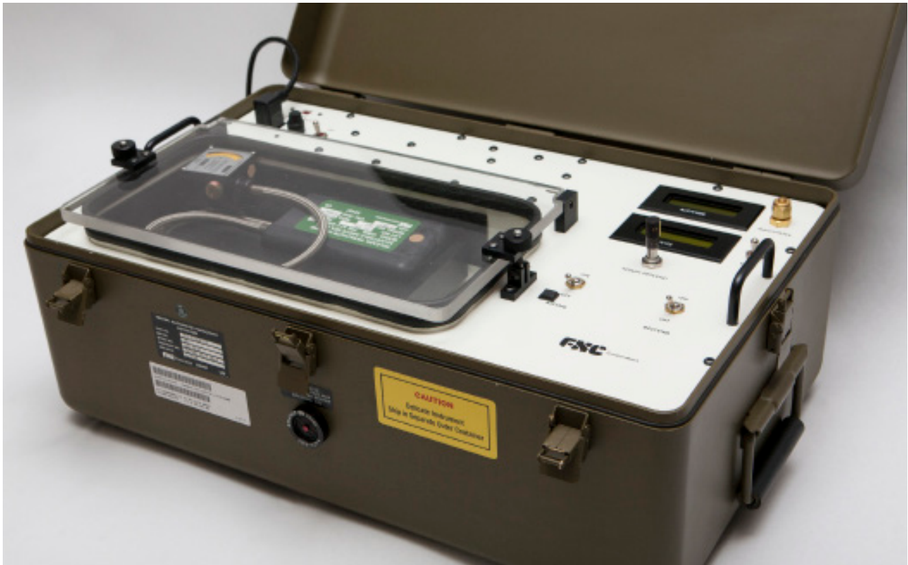
This tester is designed to test the Automatic Parachute Ripcord Release, Model 2101, FXC P/N 811-00156
